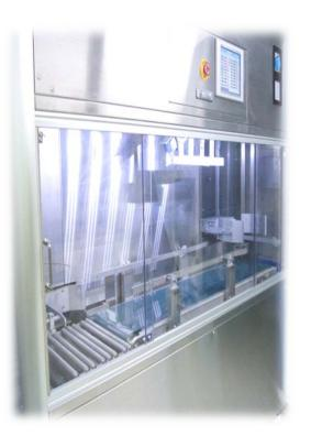
This equipment can perform entire of mineral water bottling process in one unit.
