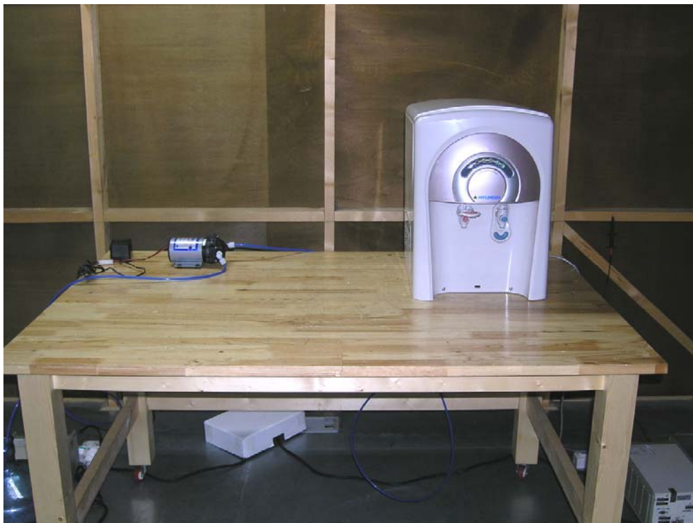
Photograph of test setup: Conducted emissions
