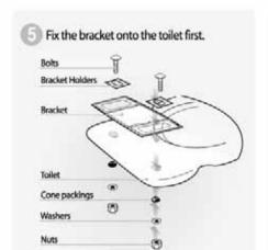
Adjust the seat and the front part of tollet back and forth so that they can correspond with before fastening the nuts.
