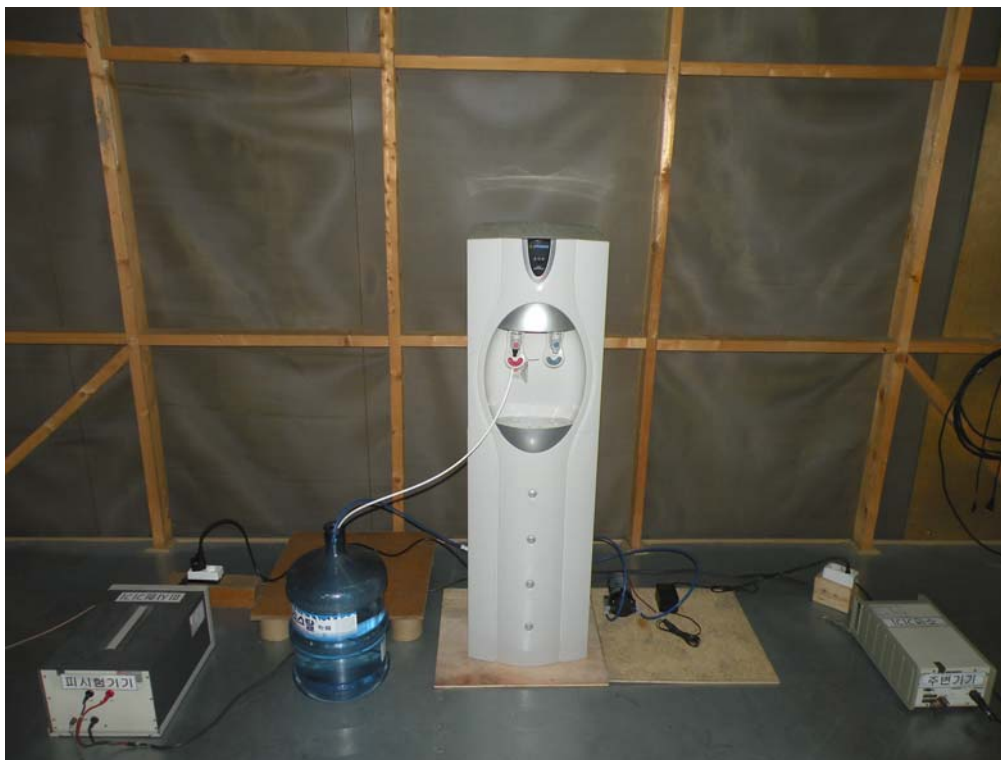
Photograph of test setup: Discontinuous Disturbance
