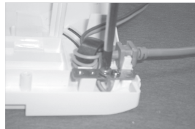
① Unloose a power cord ground line fixing bolt from the earth bracket and separate the power cord.
