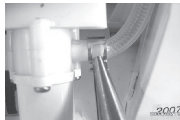
⑤ Use a tool to move the clamp inserted into the nozzle hose.
