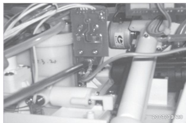
⑥ Unloose the a ground wire fixing bolt of EMI PCB at the MAIN PCB from the water tank heater bracket and separate the ground wire.
