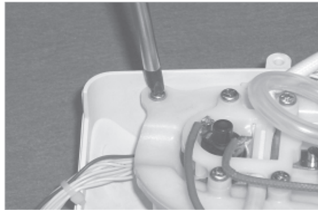
③ Unloose a water tank fixing bolt.
