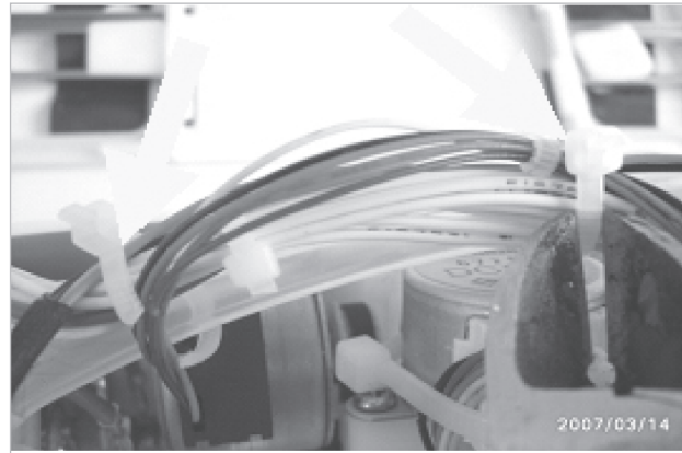
⑧ Remove 2 cable ties tightening the flow sensor at the rear base ASS'Y.
