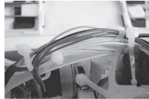
① Remove 2 cable ties tightening the nozzle stepping motor lead line.
