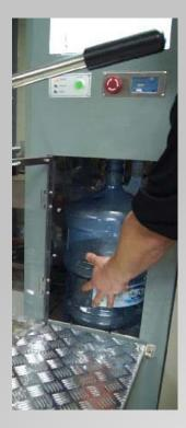
Place the bottle onto the capping machine, Open the door and push the bottle in, ( push the bottle in to the end in order to draw the bottle right up against the internal wall)
