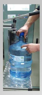
**4.** And do capping the bottle inlet port and press it by the hand,
