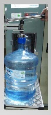
5. Place the bottle onto the capping machine and press the cap completely by the capping leva (complted)
