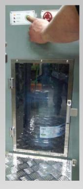
2. Close the door and press the button of "START" gently, (The filling of clean water starts when the "Filling lamp" of the front indicator lights)
