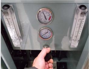
9. After fixing the operation condition, the clean water flows into the clean water tank and the concentrated water is drained through the drain pipes Now the system's operation becomes normal When tank is filled with clean water, R/O pump stops working by the pressure switch
