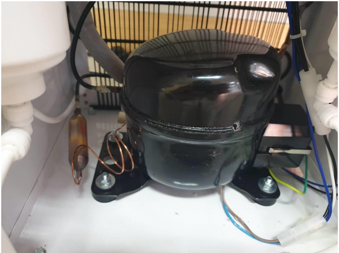
<Compressor and supply connection>
